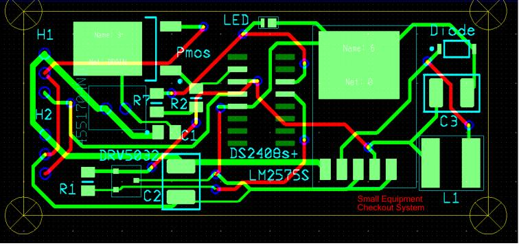
**Voltage Regulator**: Convert 12V voltage to 5V voltage to supply the DS2408 slave Device.
